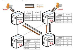
Figure 1: Overview of flat layer RADIUS server model
