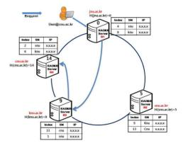
Figure 2: Overview of DHT based RADIUS server model
